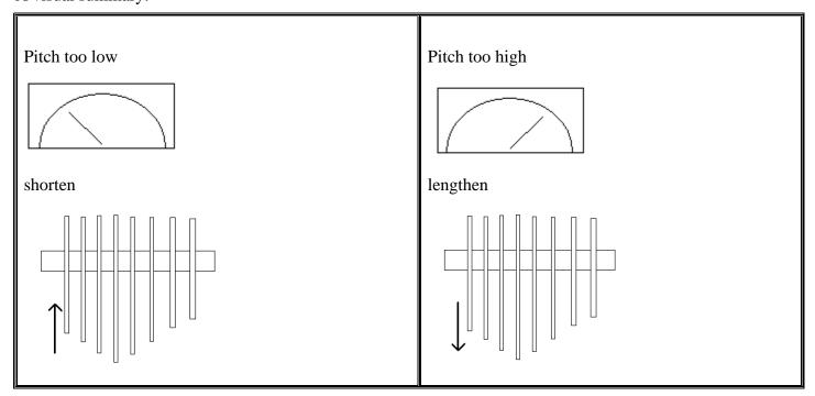
The tines near the tuner might be deadened by its being clamped to the bar. Tune tines farther away, then move the tuner.
