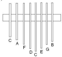
If your kalimba is already in tune and you need to disassemble it for some reason, use masking tape to hold the tines in position and remove them all as a unit. Line the tape up with something (like the edge of the bridge) so that you can get it back to the same position. Then retuning will be fairly easy.
